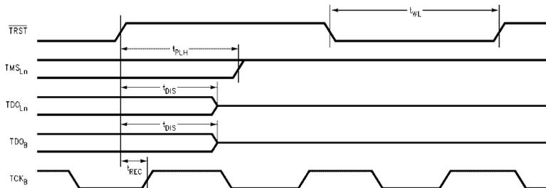
FIGURE 15. Reset Waveforms
