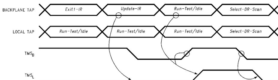
FIGURE 10. Local Scan Port Synchronization from *Parked-RTI* State
