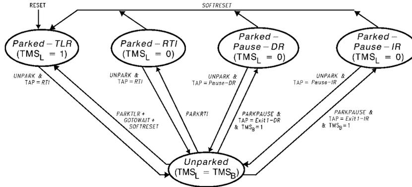
**FIGURE 4. Local SCANPSC110F Bridge Port Configuration State Machine**
