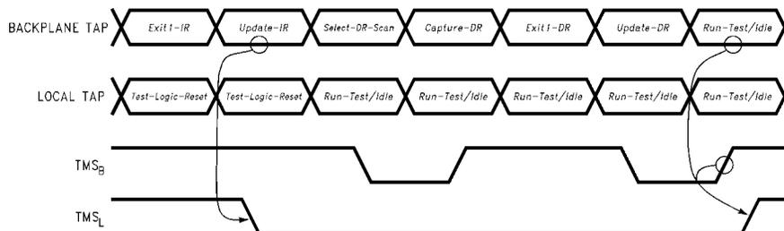
FIGURE 11. Local Scan Port Synchronization on Second Pass
