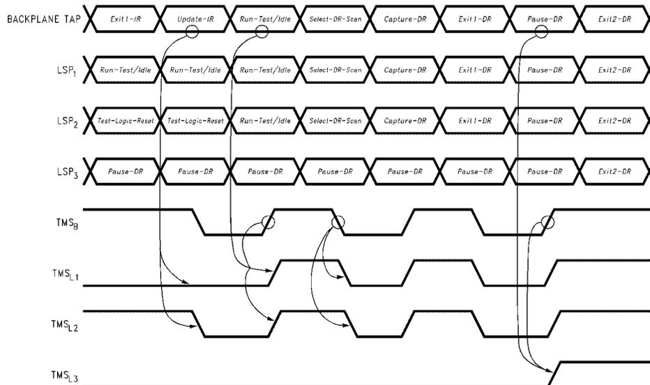
**FIGURE 12. Synchronization of the Three Local Scan Ports (LSP<sub>1</sub>, LSP<sub>2</sub>, and LSP<sub>3</sub>)**
